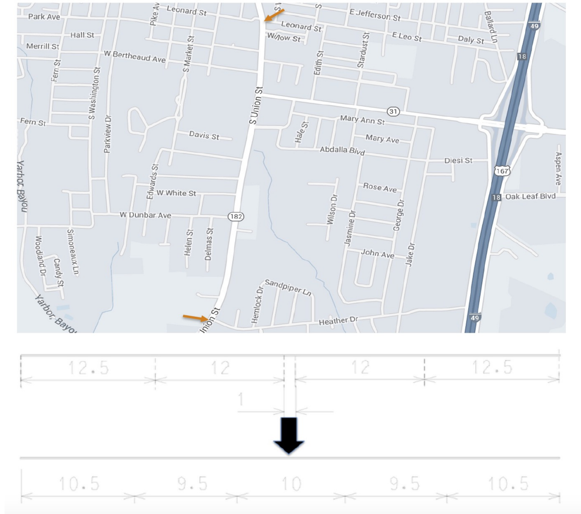
Figure 2.6. LA 182 layout and lane configuration (before and after)
